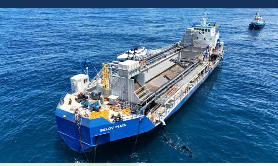
Dredge **Belov Piatã** was launched in 2024. She has a load capacity of 1640 tons for a 3120 m³/h suction capacity distributed in 4 pumps and 4 A-frames. The dredger has a length of 66.45 m, moulded breadth of 16.5 m and a draft of 2.94m. **Belov Piatã** was designed in 3D and has high quality finish.
