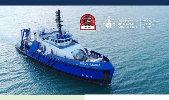
DSV designed by Robert Allan - Naval Architects and Marine Engineers (RAL). First brazilian diesel-electric diving support vessel. The DP-2 rated vessel is fitted with air diving capabilities, a light Work Class ROV and knuckle-boom crane to allow effective offshore operations. The propulsion includes three main waterjets and three tunnel thrusters, which allow safe diving conditions while divers are near the surface.
